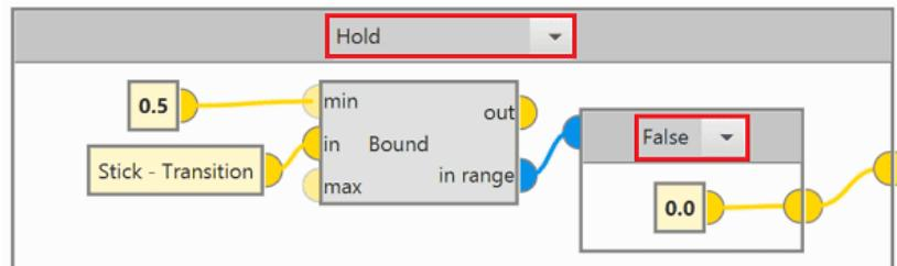
Otherwise, if the Stick-Transition variable has a value **greater than 0.5**  $\Rightarrow$  Input for Mixer block = **1.0**.
