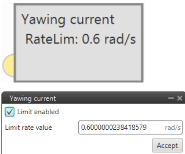
In addition, a **limit rate value** of 0.6 rad/s has been defined to control the speed at which the aircraft yaws in the guidance of this phase.
