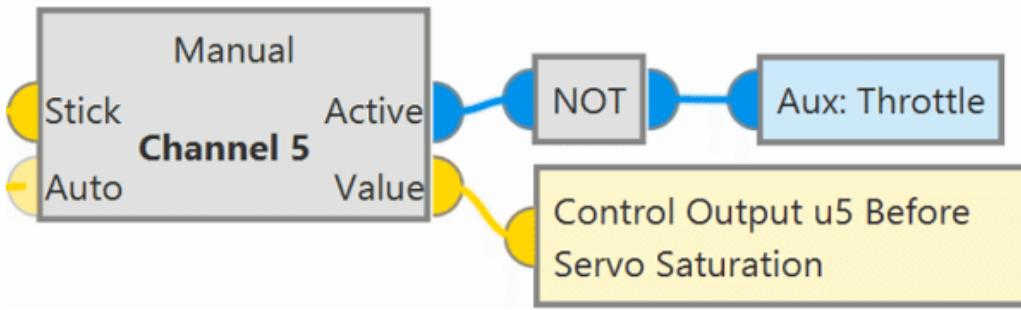
The Value output of this block must be linked to the Control Output u5 Before Servo Saturation variable, since this variable controls the actuation of the Throttle defined in the [Actuator block](#).
