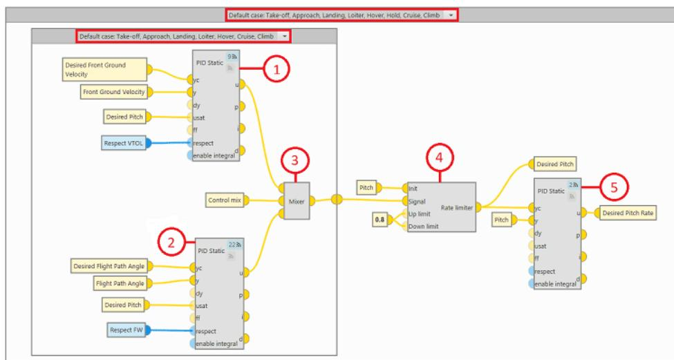
The program is basically controlled by 3 PID controllers, which provide the speed ratio as a function of the input variable and the desired variable.
