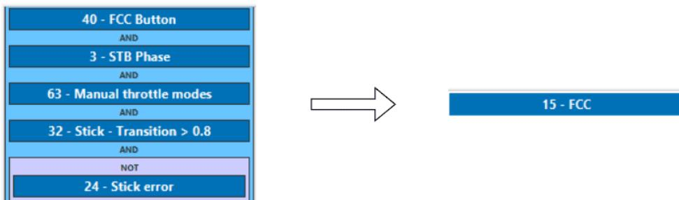
This flight phase is only performed in FW flight configuration, so the Stick - Transition variable that defines the configuration in which the aircraft flies must be greater than 0.8. This is because this variable is 0 when the configuration is quadcopter and 1 when the configuration is FW.
