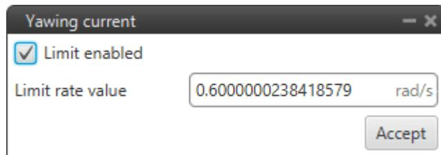
In addition, a **limit rate value** of  $0.6 \text{ rad/s}$  has been defined to control the speed at which the aircraft yaws in the guidance of this phase.
