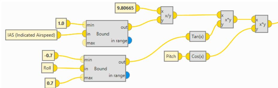
**Bound block** limits the **IAS** and **Roll** values. The minimum value for the **IAS** is  $1.0 \text{ m/s}$ , and the value for the **Roll** angle should be between  $[-0.7, 0.7] \text{ rad}$ .
