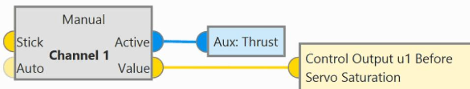
The Value output of this block must be linked to the Control Output u1 Before Servo Saturation variable, since this variable controls the actuation of the Thrust defined in the [Actuator block](#).
