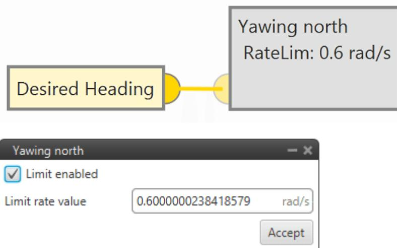
In this case, the variable Desired Heading is connected to the input, so Desired Yaw = Desired Heading.
