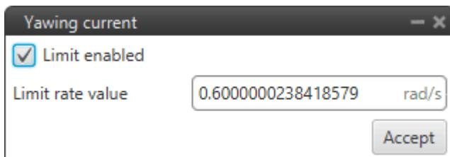
With the Yawing current block it is intended that the aircraft **maintains the yaw angle it has when entering the phase**, i.e. Desired Yaw = Current Yaw.
