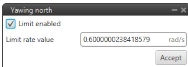
With this block it is desired that the aircraft maintains the yaw to the north (angle 0°).
